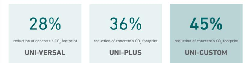
Compared with RAPID cement concrete
